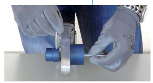
Assemble the male and female bushings on the cold plate and connect the welder to the power network. Wait for the sound or light signal (see the user's manual of the welder) that informs that the actual temperature is reached.
