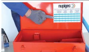
Inside Nupi Americas' welding case (where a tool is used that is supplied by Nupi Americas, this will not be true when using welding devices supplied by others) you will find a sheet that shows the welding parameters (diameter, pipe insertion depth, heating time, fusion time and time prior to testing).
